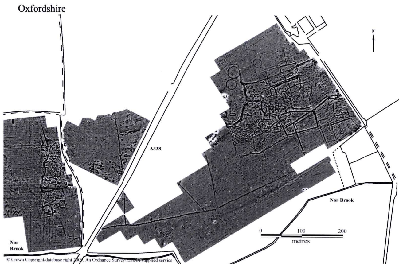
Fig 28. Geophysical Survey in Field 3 (Iron Age and Roman Settlement).
